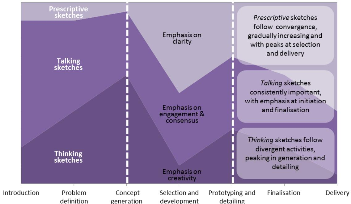
Figure 6: The use of different sketch types through the concept design phase
