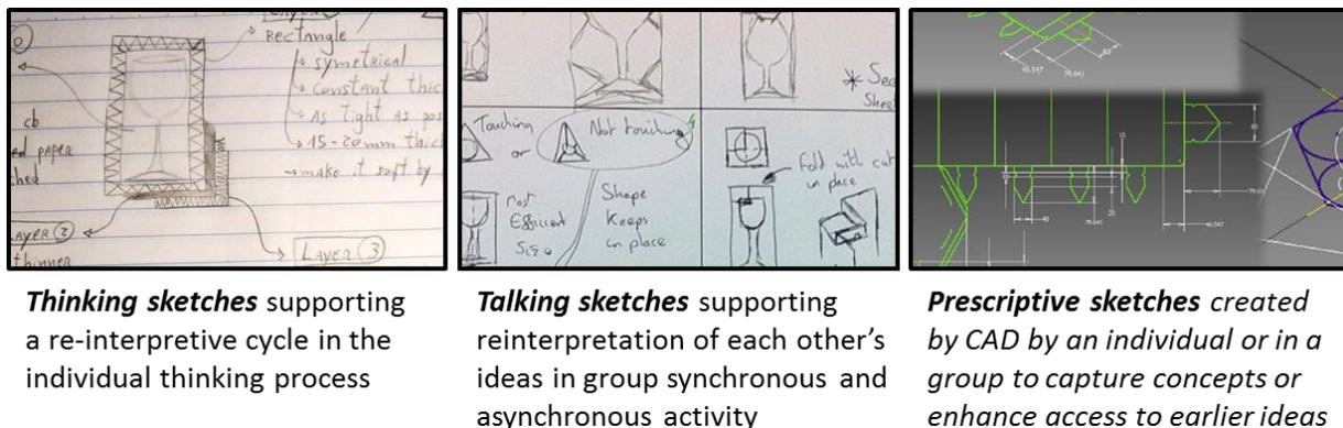
Figure 1: Types of sketches used in the conceptual design phase
