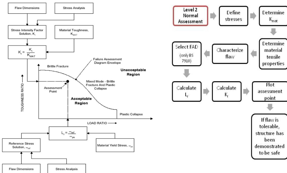
Figure 1. Overview of an FFS Analysis for crack like flaws using the Failure Assessment Diagram (FAD) – Level 2
