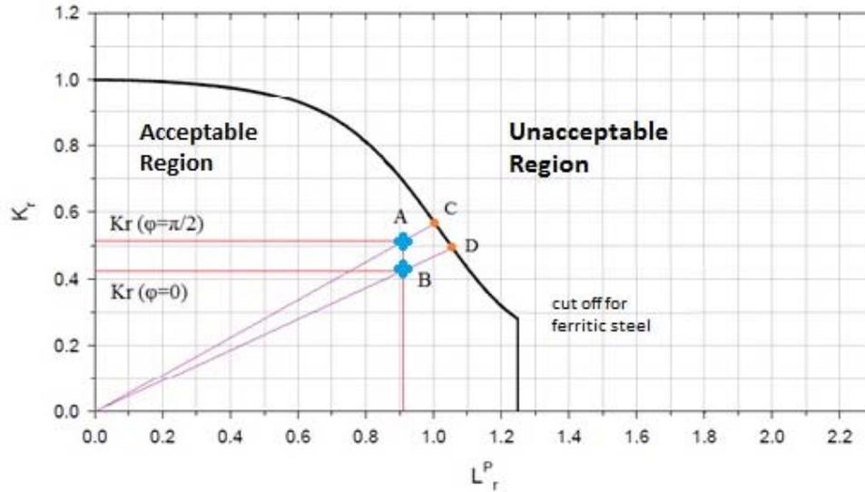
Figure 5. Assessment points using API RP 579 code
