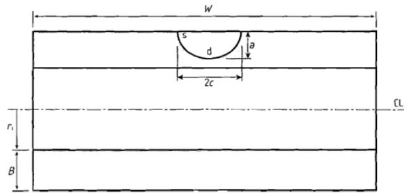
Figure 6. Section of the pipe with semi-elliptical crack-like flaw and its parameters for BS 7910
