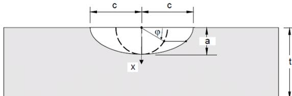
Figure 4. geometric parameters of semi-elliptical flaws
