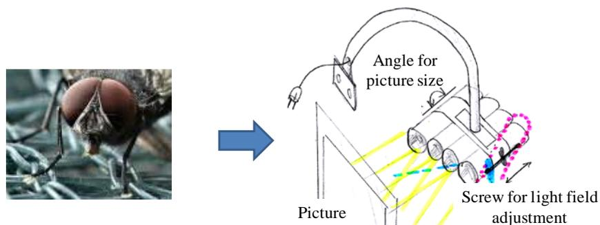
Figure 5. Lamp construction example
