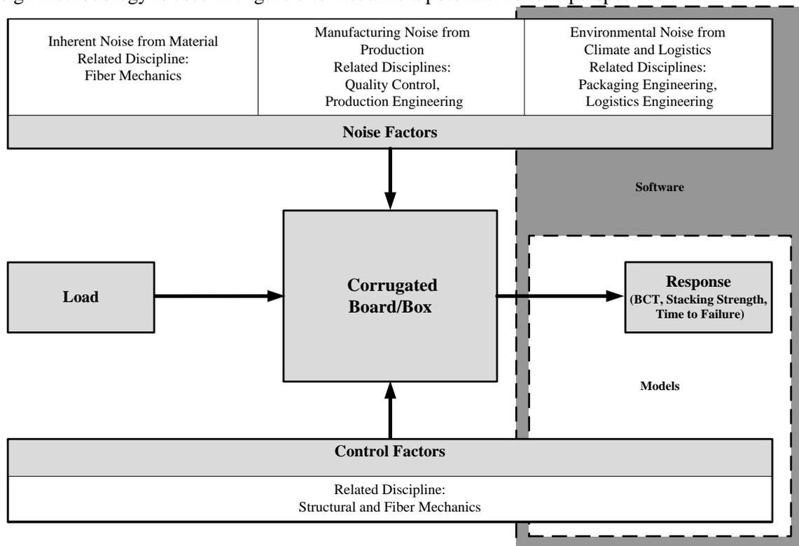
Figure 7. Holistic perspective for modeling corrugated board and box
