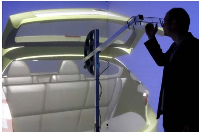
*Figure 3: Virtual real-time simulation of the physical interaction with a car back door*
