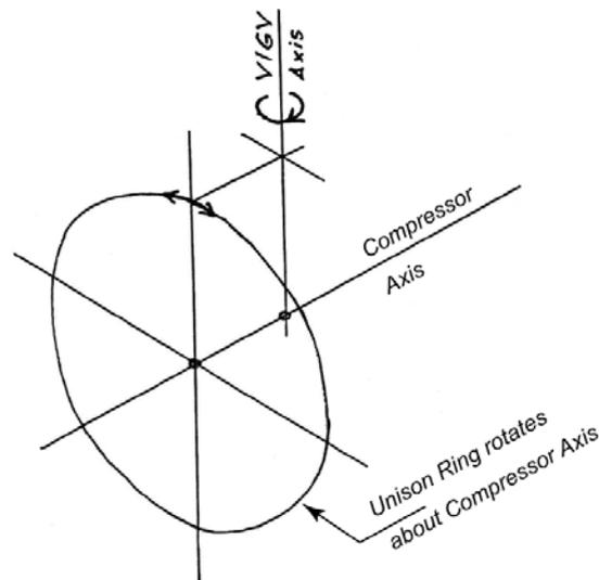
Figure 2. Schematic Diagram of Motion Requirements..
