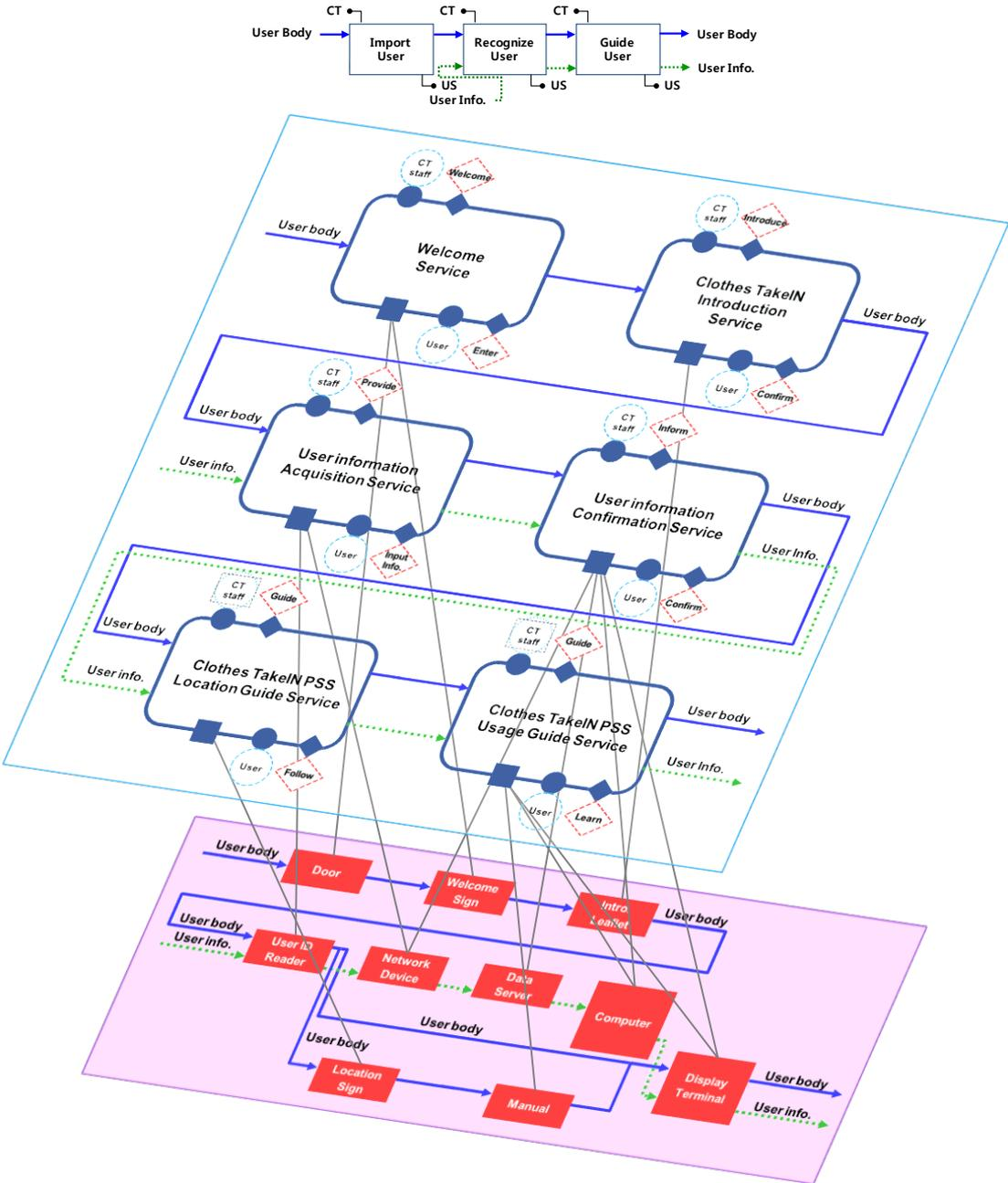
Fig. 9 PSS module representation corresponding to the function group of “Import User”, “Recognize User” and “Guide User”
