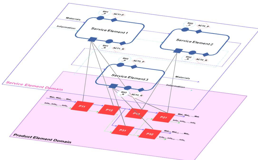
Fig. 5 3D view of PSS representation by mapping service elements and product elements
