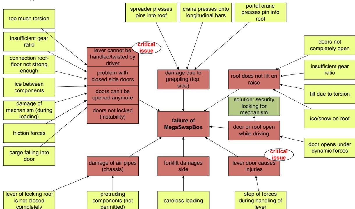
Figure 6. : Example of the analyzed fault trees
