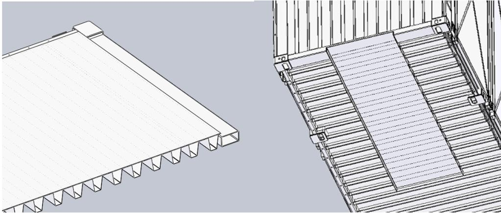
*Figure 4. Loading floor and trapeze cross member (left), Goose neck tunnel (right)*
