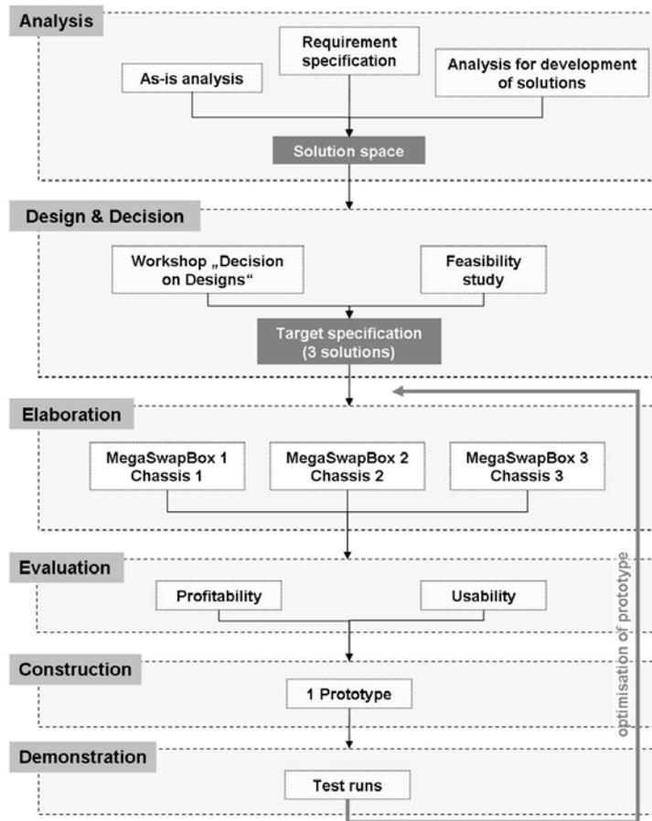
Figure 2. Methodology of design process
