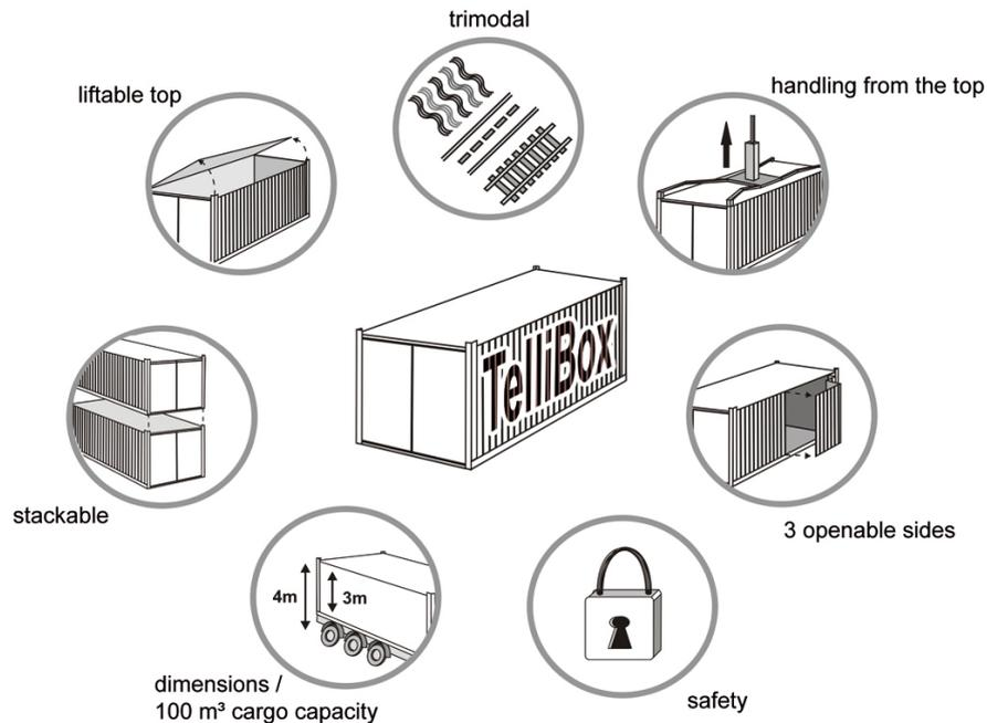
Figure 1. Requirements on the innovative loading unit
