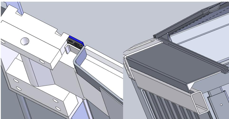
*Figure 5. Side door gadget (left), water drainage system roof (right)*
