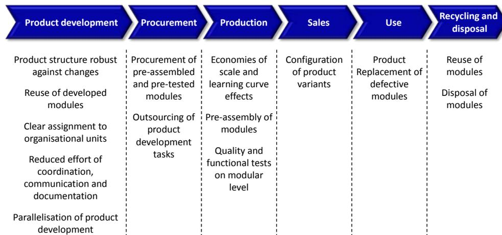
Figure 2. Advantages of modular structures for the product life phases cf. [2]
