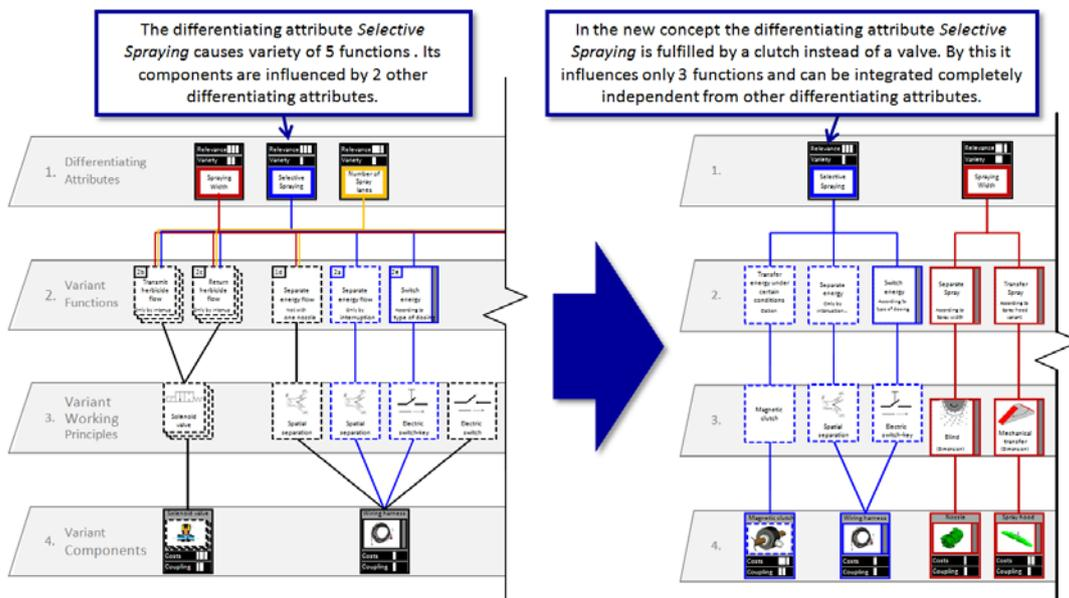
Figure 6. Applying the Variety Allocation Model (VAM) cf. [3], [11] as a tool to optimize the product family of herbicide spraying systems
