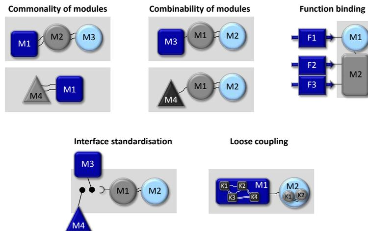
Figure 1. Attributes of modular products (F: Function, C: Component, M: Module) cf. [1]
