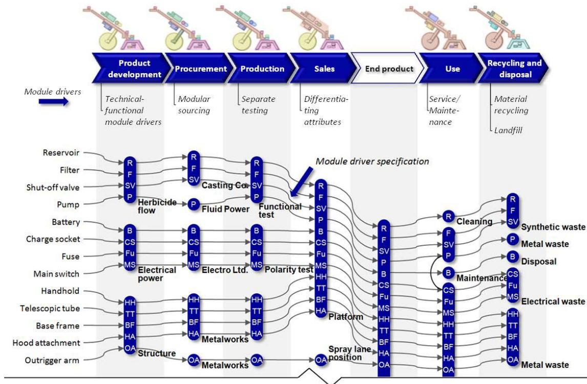
Figure 7. The Module Process Chart (MPC) as a tool to allocate module drivers and module driver specifications to modules cf. [2]
