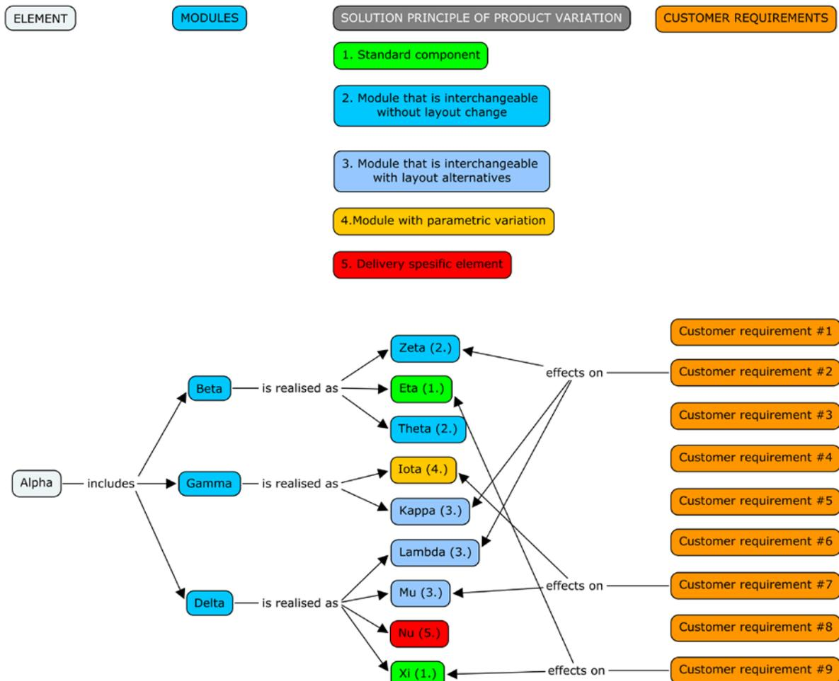
Figure 6. Product Structuring Blue Print (PSBP) for representing of module structures.
