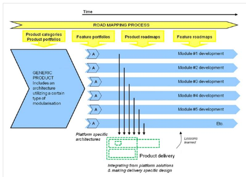
Figure 4. Dynamic Modularisation concept is a R&D method, in which everything is being developed as modules that fit into the common product range architecture. All the products are assembled from those modules. [6].
