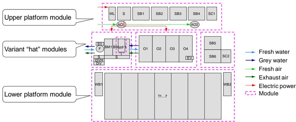
Figure 2. Module-Interface Graph (MIG) of an aircraft galley
