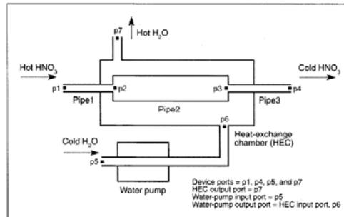
Figure 1. The structure of a nitric acid cooler [2]
