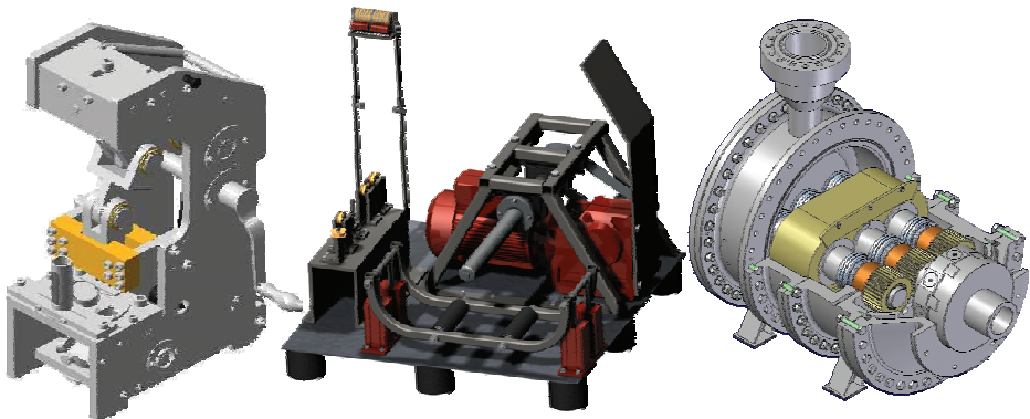
Figure 9: Examples for former design projects and typical students' solutions. Left side: a coining machine; in the middle: a wire dereeler; right side: multiphase screw pump
