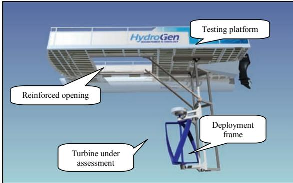
Figure 6. CAD model of test facility
