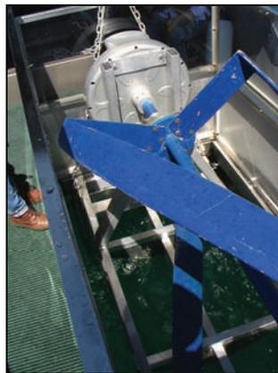
Figure 7. Helical turbine and submersible generator ready for testing.
