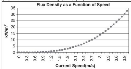
Figure 1. Energy Flux density as a function of speed [20]
