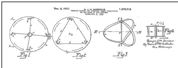
Figure 4. Darrieus turbine as filed for US patent [9]
