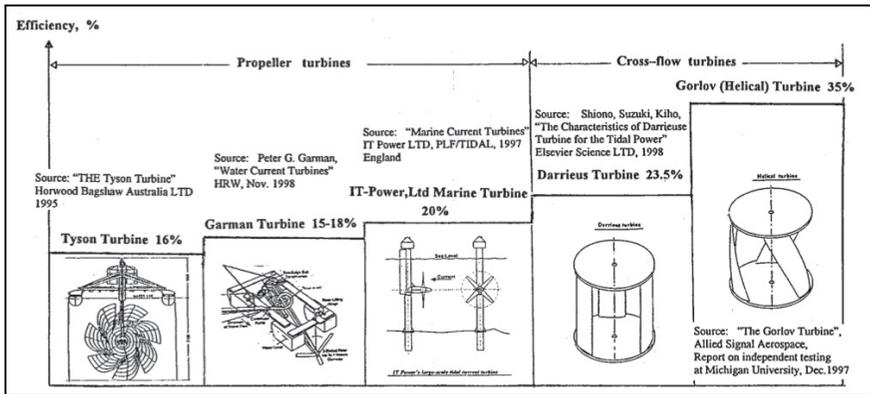
Figure 5. Comparison of turbine efficiencies [9]
