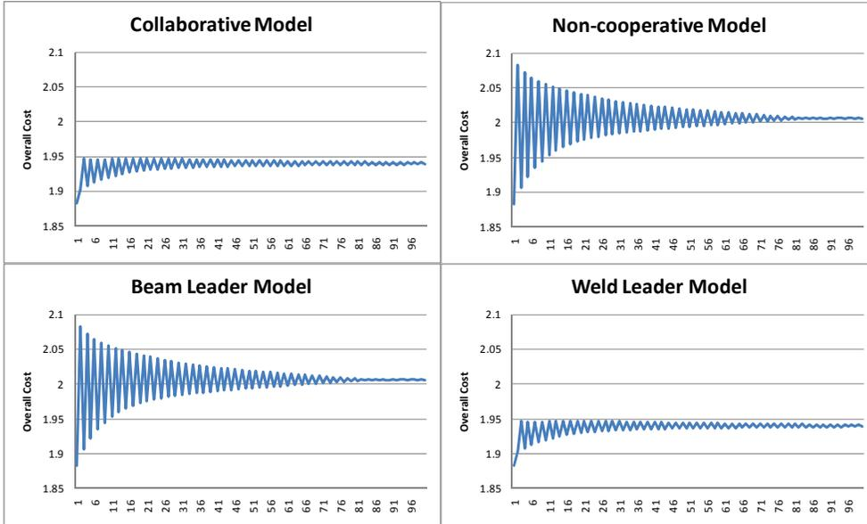
Figure 4. Plots of four interaction models in the welded beam design
