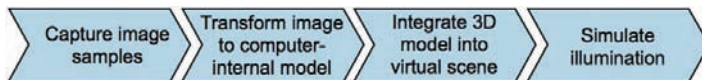
Figure 5. IBL process for the simulation of realistic illumination from sample of images, according to Debevec [3]
